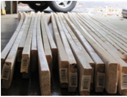
Warped furring strips. Quite frightening!
